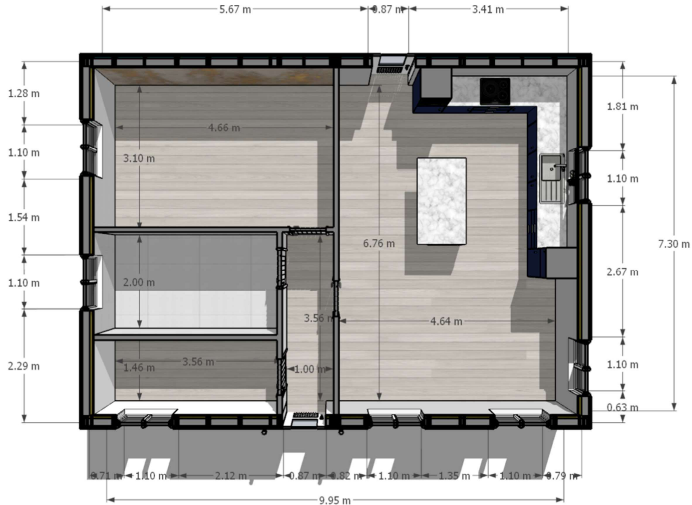
FLOOR PLAN 03 – EXTERNAL & INTERNAL DIMENSIONS
