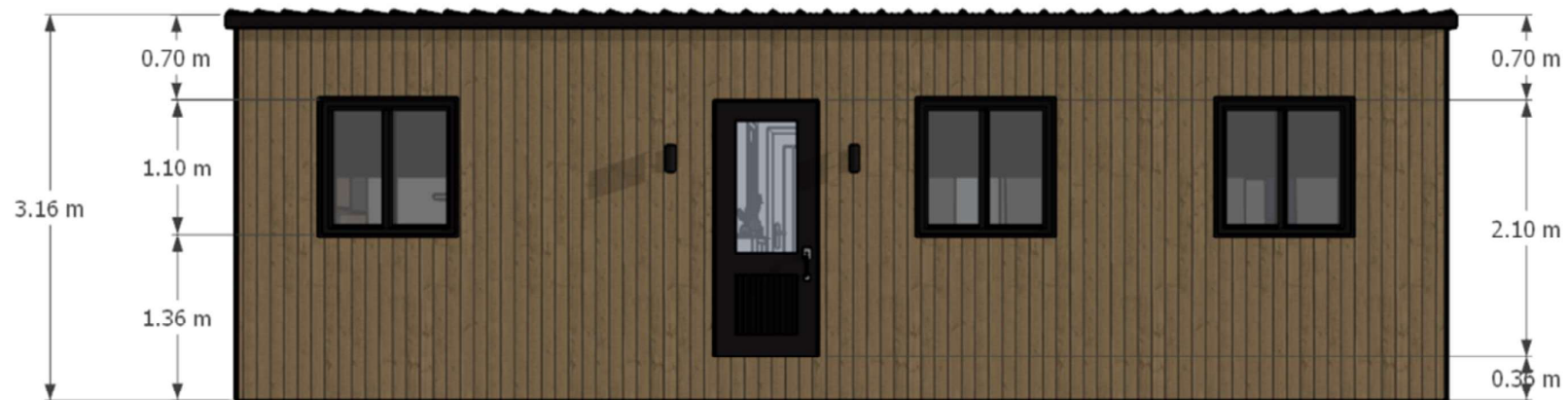
FRONT ELEVATION W/ DIMENSIONS
